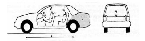
93cm/36" min. Α Cushion not compressed. В 96cm/37" min. Seat fully rearwards. C 61cm/41" min. Front seat fully rearwards. D 84cm/33" min. Cushion not compressed. Wheelbase Ε 245cm/96" min. F1 133cm/52" min. Interior width between doors F2 122cm/48" Between armrests G 25cm/10"
